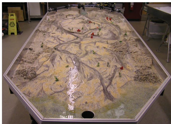
(d) A stream of water flowing over sand can simulate the evolution of a river.
